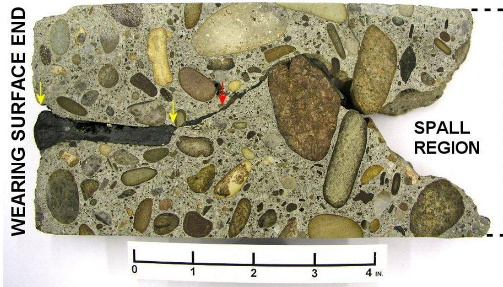
Figure 8. Lapped surface view perpendicular to the plane of the wearing surface in the Gallia County, Ohio SR 7 joint core. This is the original joint that was placed in 1946.
