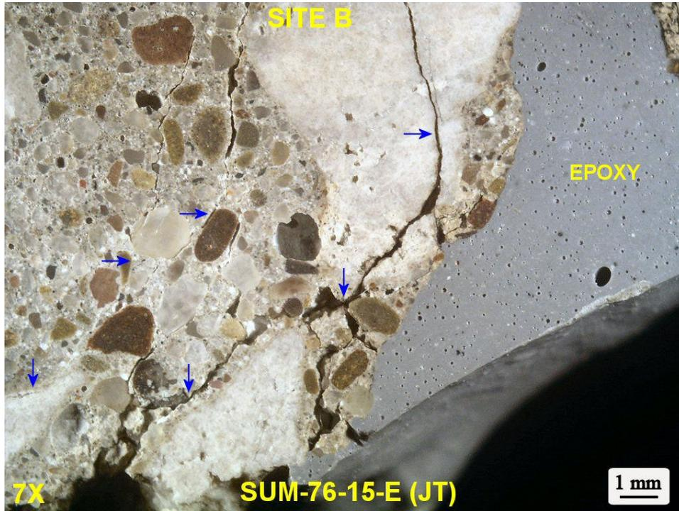
Figure 6. Enlarged view (7X) of the lapped surface of the I-76 core at Site B in Figure 4 (along the bottom end surface of the core).
