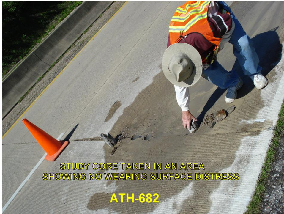
Figure 2. Joint coring sites along a transverse control joint on PCC pavement on SR 682 in Athens County, Ohio (placed in 1976, photographed in 2009).
