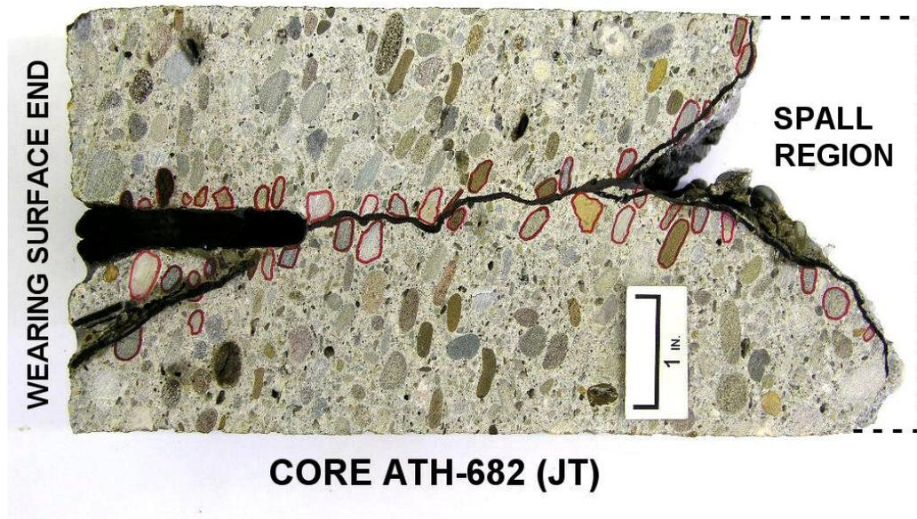
Figure 3. Saw-cut surface of the joint core taken from State Route 682 in Athens County, Ohio in 2009.
