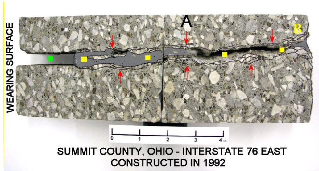
Figure 4. Lapped surface of the joint core taken from Interstate 76 East in Summit County, Ohio, showing sub-surface cracking and spalling distress.
