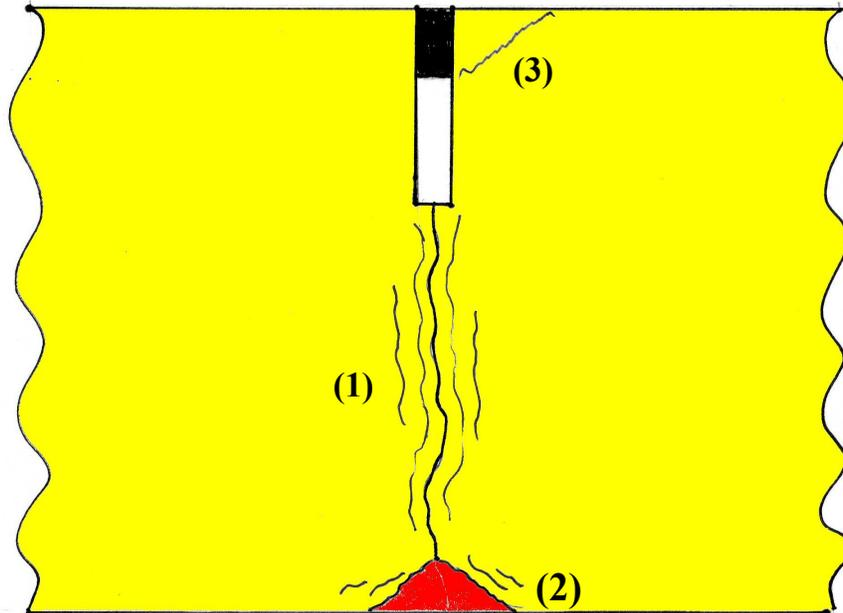
Figure 1. Schematic of the type of cracking exhibited by the joint and mid-slab crack cores examined in the present study (not to scale).
