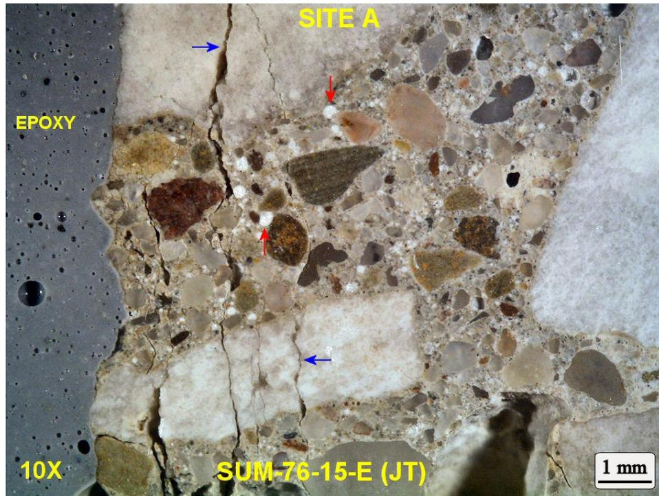
Figure 5. Enlarged view (10X) of the lapped surface of the I-76 core at Site A in Figure 4. The wearing surface is at the top in the photograph.
